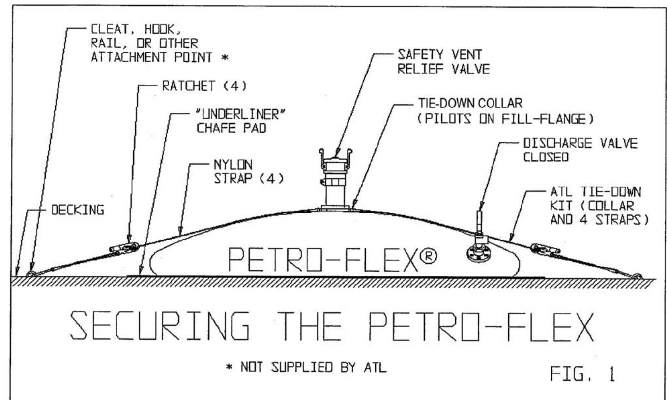
**ATL Tie-Down Collar with ratchet straps at 4 equally spaced points.**
