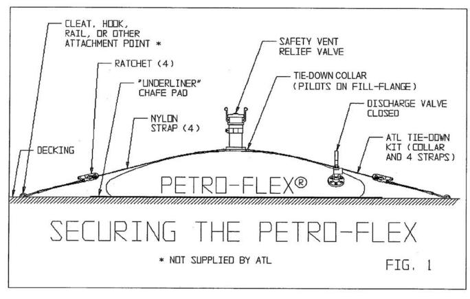
ATL Tie-Down Collar with ratchet straps at 4 equally spaced points.
