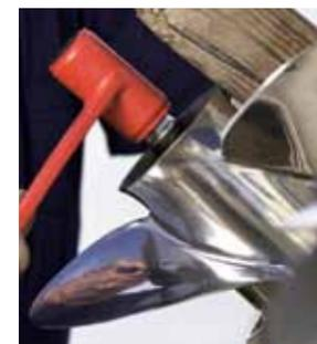
**1 PROPELLERS** Having the right propeller can make a big difference in improving your boat's fuel economy. In general, you want a prop that allows the engine(s) to rev up as high as possible and still remain within its rpm range. Try a variety of props, including three- and four-blade models, to find out which one works best for your boat.
