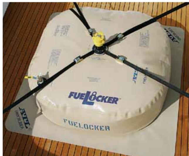
**Transferring Fuel** A fuel-outlet valve with a fuel hose lets you access the fuel. Some boaters tie into their main fuel line. This way you can burn the fuel bladders first to get them out of the way, but you have to redo your fuel lines. Also, this doesn't lend itself well to the complexity of marine diesel fuel systems, which have return lines.
