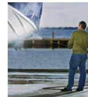
**3 BOTTOM** A boat with a clean, smooth bottom will reward its owner with enhanced efficiency. Remove old cratered layers of anti-fouling paint and recoat with an abrasive paint that will maintain a smooth surface. Drag increases as an exponent of speed, so even minor imperfections count.
