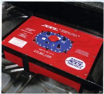
CLOCKWISE FROM UPPER LEFT: The cell itself is housed in a steel container, and we bolted this can to our support structure. We formed our frame from castoff angle steel, adding gussets wherever possible before spray-bombing it black. The rest of the cell—including the bladder, safety foam, check valves and top—could then be installed. When suspending a cell, be sure to leave enough ground clearance. If we ever lose a wheel, the cell won't be the first thing to touch the ground.
